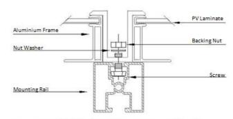
Figure 12: Detail of a top-down clamp mounting attachment
