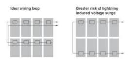
Figure 4: Wire loop design recommendation
